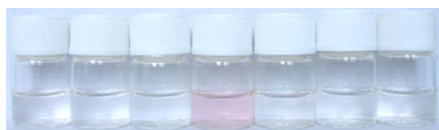
Fig. 2 Photograph of 50 μM R6GH in the presence of different of the nitrate salts (10.0 equiv) of ClO 4 - , H 2 O 2 , NO 2 - , ClO - , TBHP, Cu 2+ and Hg 2+ in H 2 O
